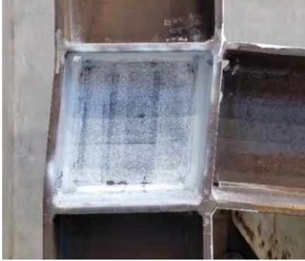
Figure 5.5: W250-NDP at the end of the test at 0.12 shear strain: (a) Deformed shape, (b) DIC shear strain contour (shear yielding \gamma_y = 0.007 is shown by the boundary of purple and blue – red represents maximum strain)
