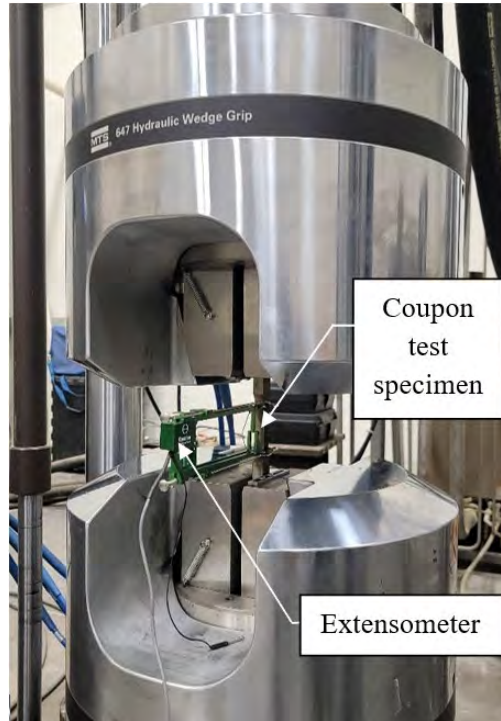
Figure 4.18: Uniaxial load frame used to perform standard coupon tests
