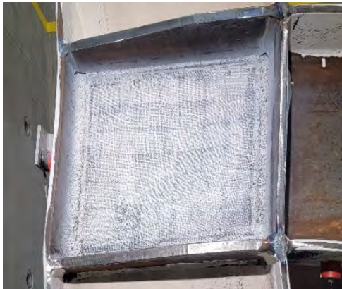
Figure 5.11: W410-RDP1A at the end of the test at 0.12 shear strain: (a) Deformed shape, (b) DIC shear strain contour (yielding \gamma_y = 0.008 is shown by the green areas – red represents maximum strain)
