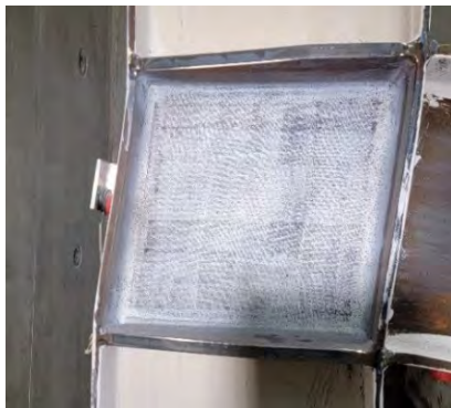
Figure 5.6: W410-NDP (Column web Face 2 is shown) at the end of the test at 0.12 shear strain: (a) Deformed shape, (b) DIC shear strain contour (shear yielding \gamma_y = 0.008 is shown by the boundary of purple and blue – red represents maximum strain)
