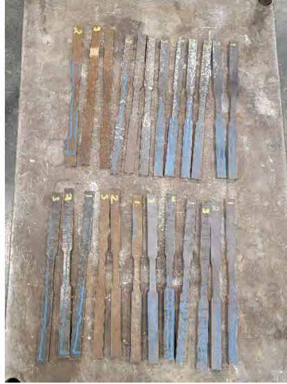
(a) Coupon specimens before testing
