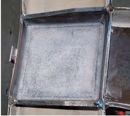
Figure 5.12: W410-RDP1B at the end of the test at 0.12 shear strain: (a) Deformed shape, (b) DIC shear strain contour (yielding \gamma_y = 0.008 is shown by the green areas – red represents maximum strain)
