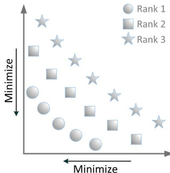
Figure 3-8: Illustration of non-dominated sorting with the population divided into three ranks (Tian et al., 2017)
