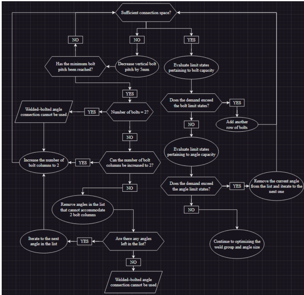
Figure 4-11: Flowchart of second step of the optimization procedure of welded–bolted angle connections
