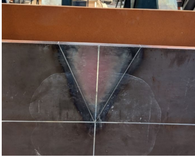
Figure 3-22: Vee heat on the damaged specimen at the desired temperature
