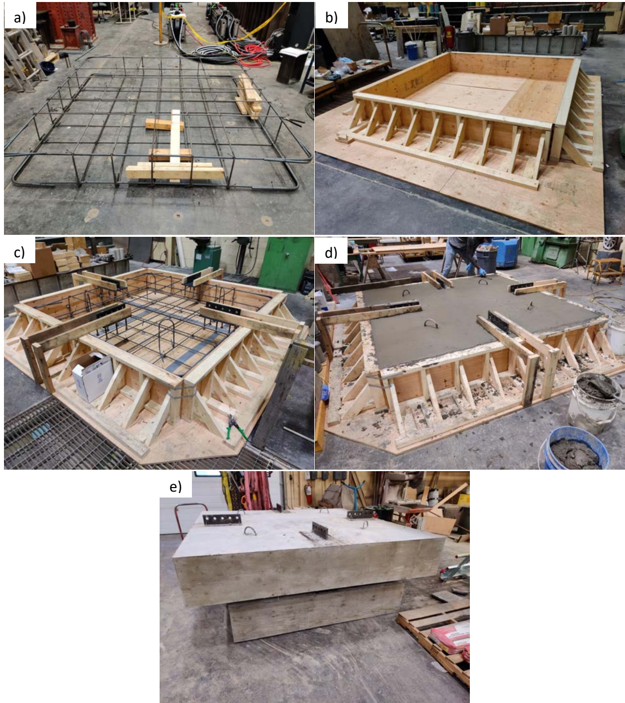
Figure 4.4 Specimen fabrication process (a) reinforcement cage, (b) formwork, (c) formwork (immediately before pouring), (d) casting/finishing concrete, (e) finished concrete specimens
