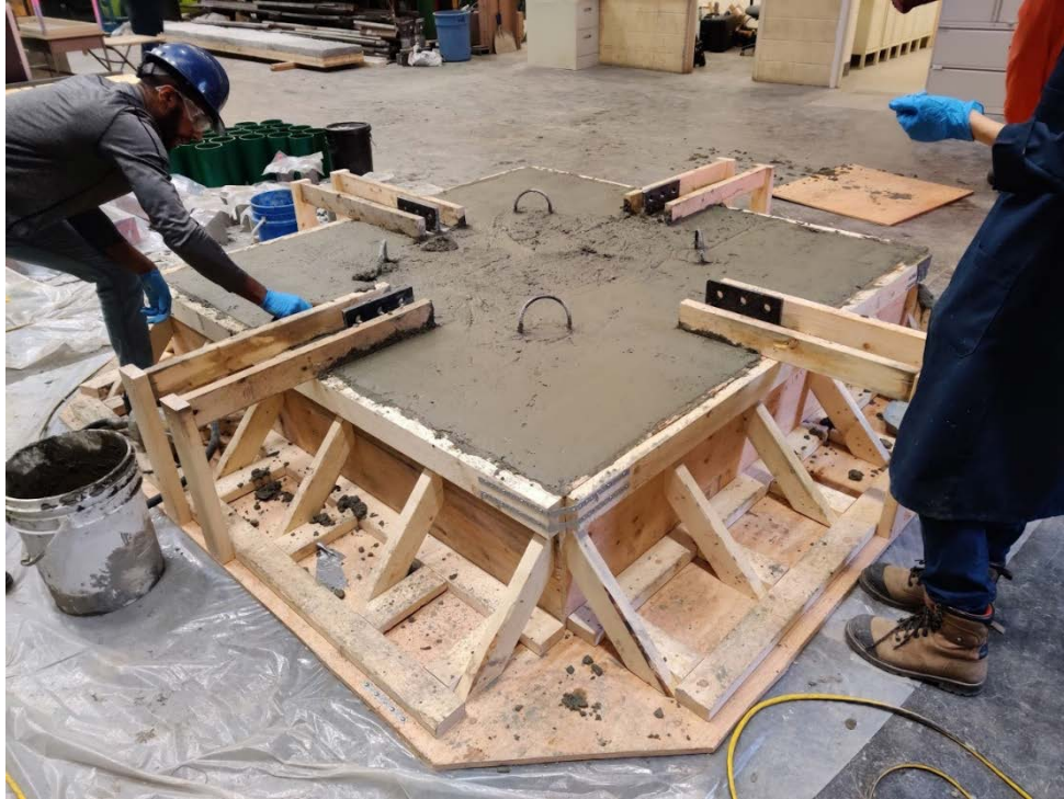
Figure D.5 Finishing of SEP4 concrete specimen
