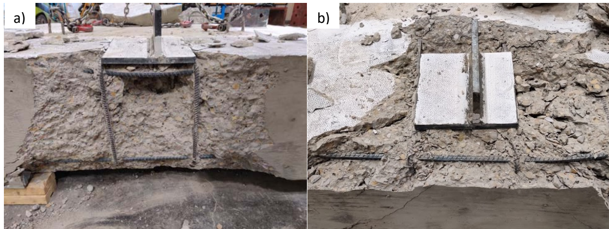
Figure 4.10 Edge reinforcement after testing of (a) SEP4-150-125 and (b) SEP4-150-175
