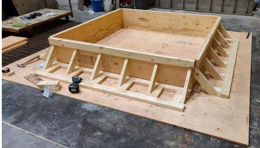
Figure D.1 Formwork for SEP4 concrete specimen
