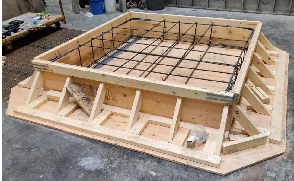
Figure D.3 Placement of reinforcement into SEP4 concrete specimen formwork
